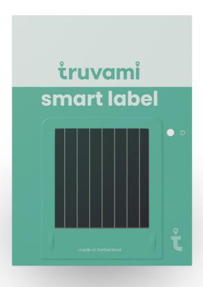
truvami® smart label is a powerful, seamless indoor/outdoor tracker offering precise localization with minimal energy consumption. It integrates a multi-standard GNSS receiver, passive Wi-Fi MAC address scanner, and sensors such as an accelerometer, temperature/humidity, and pressure sensor, all within an ultraslim, flexible form factor. Fully autonomous, the device is completely battery free, powered entirely by ambient light through OPV technology, and can even last for weeks without light.
